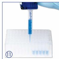
Stepper™ is best suited for dividing samples in small portions, for precise dispensing in tubes and vials or screening procedures.
