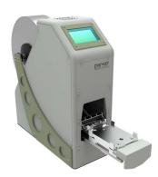
The Ultraseal™ XT-PRO unit is an automated heat applied microplate and tube rack sealer. The unit uses a roll of surface modified aluminium or plastic film approx. 78mm wide and 610mm long, positioned to the rear of the sealing section.
