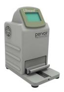
The Ultraseal™ LITE is a semi-automated heat-applied microplate and tube rack sealer. The unit uses pre-cut sheets of surface modified aluminium or plastic film, approximately 78mm wide and 130mm in length, applied to the plate top surface to create the seal between plate and film.
