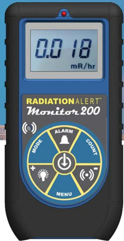
The Monitor 200 measures alpha, beta, gamma, and x-rays. Its digital display shows readings in your choice of CPM, CPS,  $\mu\text{Sv/hr}$ , mR/hr, or in accumulated counts. It has a red count light, and a beeper that sounds with each count detected. Other features include an adjustable timer, and selectable alert. With the free Observer USB Software Family, you can set computer alarms, calibrate your instrument, and download your collected data from the internal memory for easy reporting!
