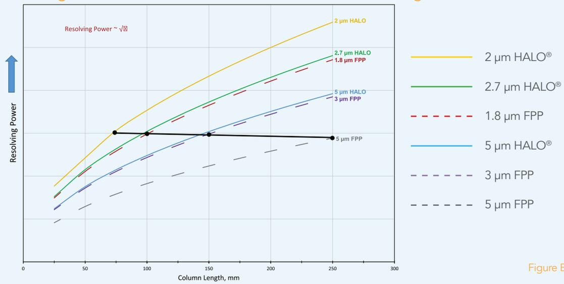
**Example 1:** A 100 mm column packed with 2.7  $\mu\text{m}$  HALO<sup>®</sup> particles meets the criteria of providing equal or better resolving power compared to a 250 mm column packed with 5  $\mu\text{m}$  FPP particles. The HALO<sup>®</sup> column is an appropriate choice for replacing the 250 mm length FPP column in an ultra-fast method.
