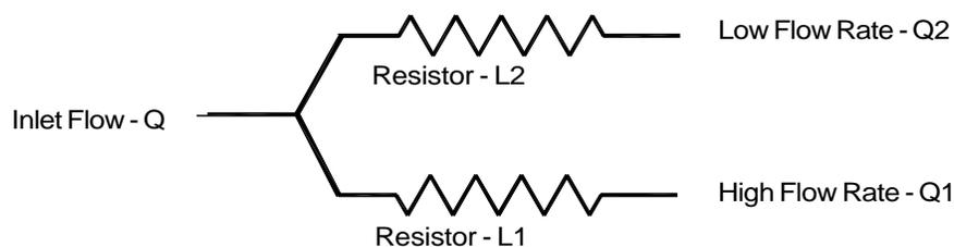
L1 = Fixed fluid resistor (resistance value varies depending on cartridge rating)
