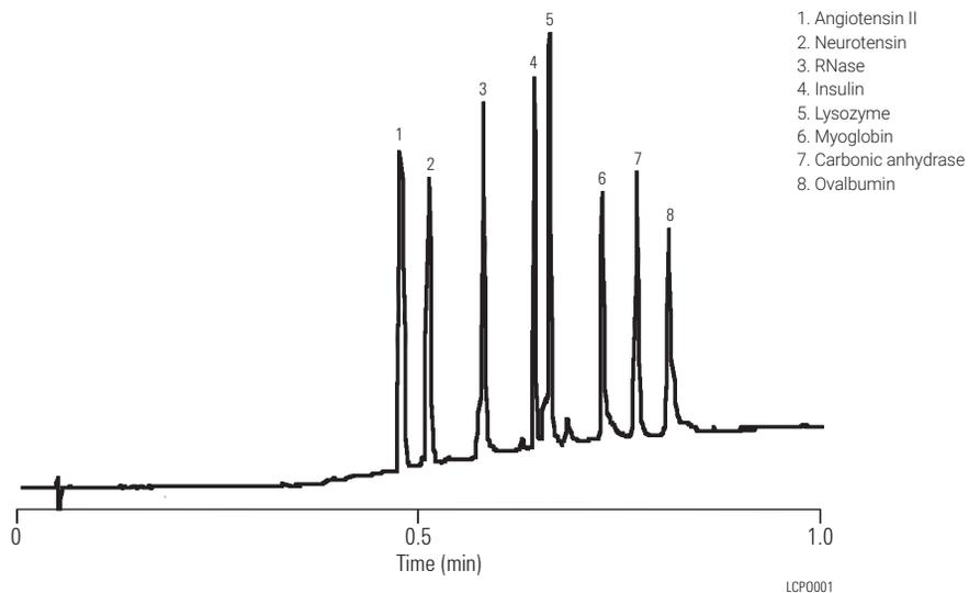
This separation of eight polypeptides and proteins is completed in less than 60 seconds. Each peak is sharp and efficient.
