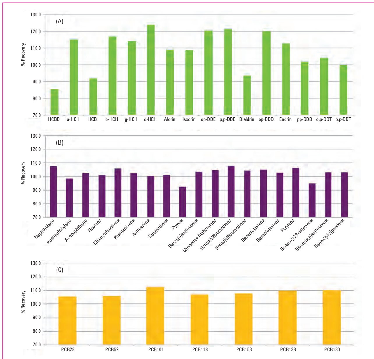
Figure 3. Graphical representation of analyte percent recovery values for (a) OCPs, (b) PAHs and (c) PCB congeners in spiked mussel tissue.
