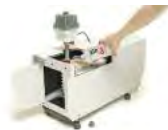
Adding foreline pump (rotary pump) oil, 4 L
