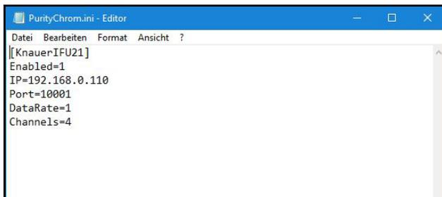
**Fig.3** Configuration example for IFU 2.1 LAN
