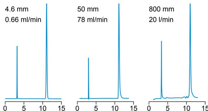
All Kromasil pre-packed columns are delivered with a minimum performance guarantee of at least 40 000 pl/m for 10 µm particles. For larger diameters DAC columns are recommended. The performance obtained in analytical columns can be maintained all the way up to very large industrial scale DAC columns, and in the example an 80 cm ID DAC column is proven to show analytical performance. The scale-up factor from the analytical column in this case is 30 000 times.
