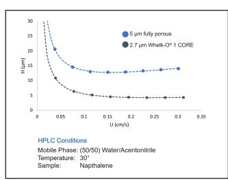
WHELK-0 $^{\circ}$  1 Core provides higher column efficiencies than similarly-sized fully porous particles, even at higher mobile phase linear velocities. H vs U curves compare performance of 2.7  $\mu$ m WHELK-0 $^{\circ}$  1 Core and 5  $\mu$ m fully porous WHELK-0 $^{\circ}$  1.
