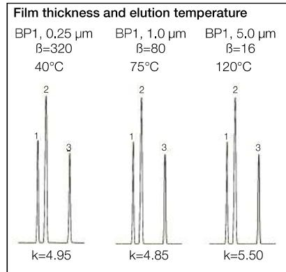
As well as film thickness, changing the column internal diameter also effects the elution temperature. To avoid using two parameters that can alter individually, phase ratio is often used as it takes both into account.
