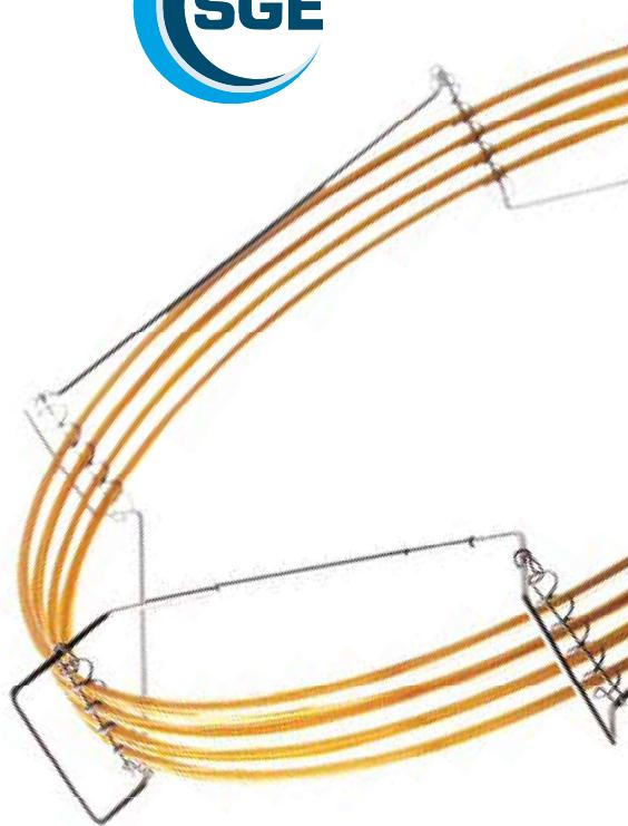
There is also a minimum temperature below which a column will perform poorly. If a column is run continuously at the upper limit of temperature, column bleed will be observed. This is background noise caused by stationary phase degradation and this increases with increased film thickness.
