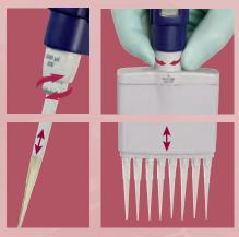
The multichannel bowed shape ejector head permits effortless, sequential tip ejection.
