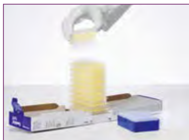
② Lift transfer cover. Tips fully protected.
