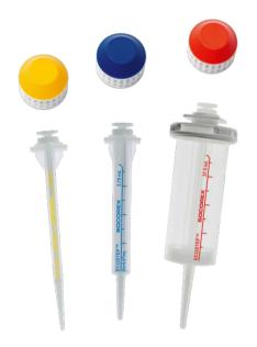
Three syringe sizes cover full volume range from 10 to 5000 µL. Colour coding on syringe and selector button eliminates any setting error. The graduation helps monitoring syringe content. Available in standard non-sterile and sterile bioproof ™ versions. Compatible with all Stepper™ generations.
