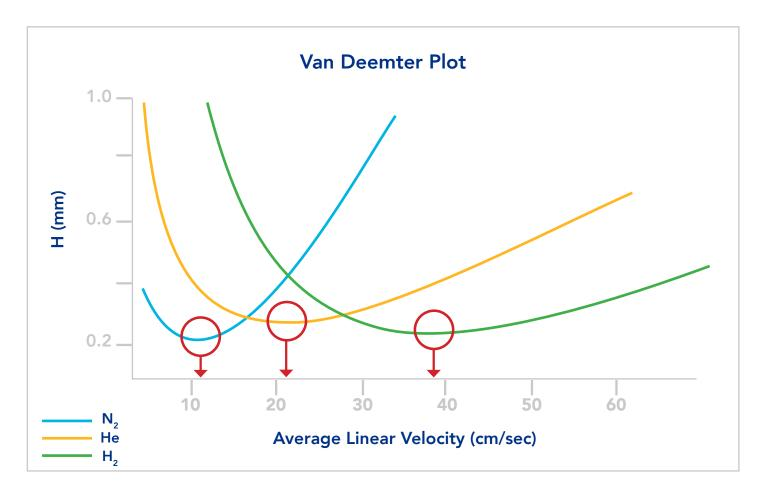
Hydrogen can be used as an effective replacement for helium in most GC and GC/MS applications. It has a wide range of applicability, provides good efficiency and separations are faster than helium.
