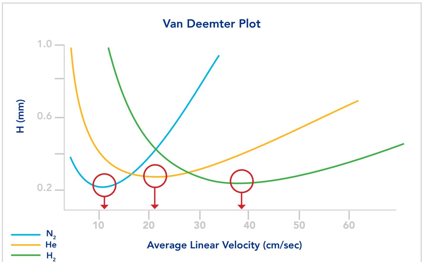
Hydrogen can be used as an effective replacement for helium in most GC and GC/MS applications. It has a wide range of applicability, provides good efficiency and separations are faster than helium.
