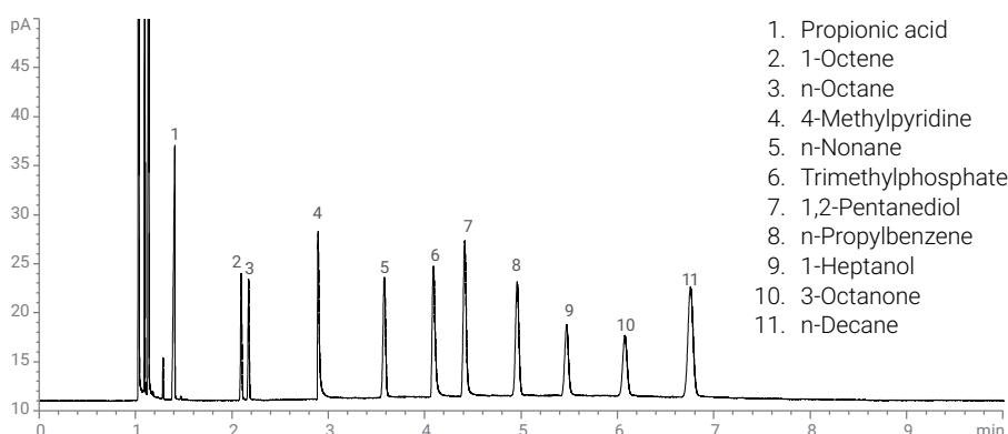
Every Agilent J&W 5Q column is tested with our demanding Über One test probe mixture to ensure consistent, reliable performance for challenging active analytes.
