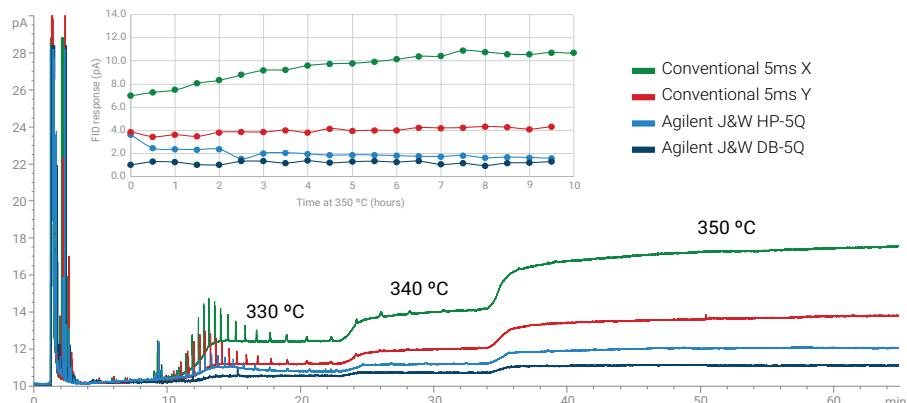
Compared to conventional 5ms columns, Agilent J&W 5Q GC columns have significantly lower bleed profiles, resulting in more stable baselines. A more stable baseline ensures accurate integration, especially for trace-level analytes with low signal-to-noise ratios.
