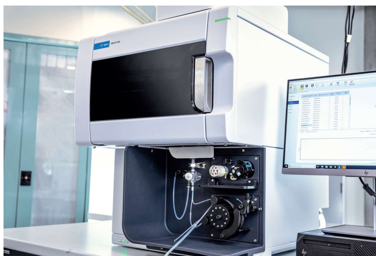
Agilent 5900 ICP-OES can be used to run EPA 200.7 methods
