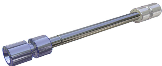
Figure 3: Schematic of sample tube fitted with two DiffLok caps, ready to be placed in an automated thermal desorber. The cap at the sampling end of the tube (on the left) is inert-coated stainless steel, whereas the cap at the non-sampling end (on the right) does not encounter the flow of analytes and so is regular stainless steel.
