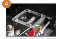
**Analysis:** The trap is thermally desorbed at up to 100°C/s to inject the sample into the GC-MS as a narrow band.
