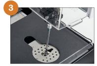
**Probe desorption:** The probe is thermally desorbed and vapours transferred to the focusing trap.
