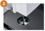
**Probe washing:** The probe is removed from the vial and a wash/dry station removes residual sample matrix.
