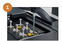
Probe insertion and analyte extraction: The robot inserts the probe into the vial, and the assembly is incubated/agitated to ensure analyte equilibration.
