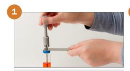
**Probe insertion:** Two probe lengths allow immersive or headspace sampling in 20 or 10 mL yials.
