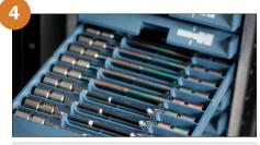
**Probe desorption and analysis:**Probes are inserted into industrystandard tubes for analysis by TD-GC-MS.
