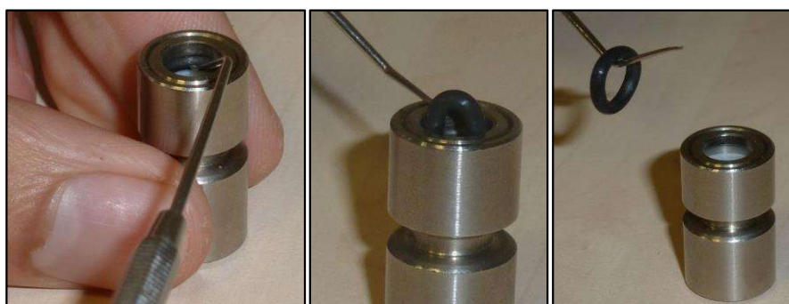
Figure 3: How to remove o-ring from DiffLok cap
