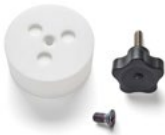
The components of the \mu -CTE chamber calibration tool.
